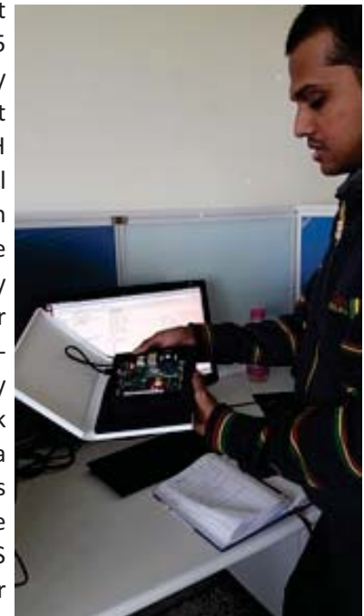
Figure: Post Doctoral fellow Dr. Asan Basiri working on a cryptographic co-processor development on a Xilinx FPGA based prototyping environment
